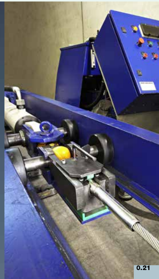
↑ Inox-Seil WC Câble Inox WC Stainless steel wire rope WC 6 x 19 + WC E = 1,0 - 1,3 \cdot 10^5 \text{ N/mm}^2
