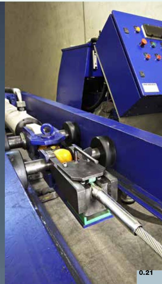
↑ Inox-Seil WC Câble Inox WC Stainless steel wire rope WC 6 x 19 + WC E = 1,0 - 1,3 · 10 5 N/mm 2
